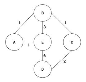
(1) E begins to calculate its shortest paths to all other routers. Fill in the following table that contains routing information for E. Columns represent destination routers. You may use any shortest path algorithm (i.e. Dijkstra's) to calculate shortest paths.
