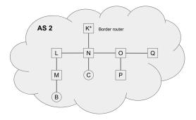
For this question, K is AS2's single border router connecting to all other ASes from question 2.1. Assume that internally, AS2 is running the learning switch algorithm for IGP. All routers in the network start with empty forwarding tables.
