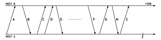
The above figure shows the life cycle of a TCP connection with normal termination - that is, connection establishment, data exchange, and teardown.
