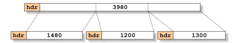
Must reassemble to recover original packet
