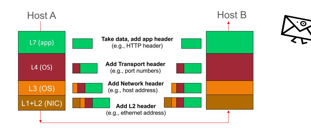
Packets, headers, header encap/decap at different points
