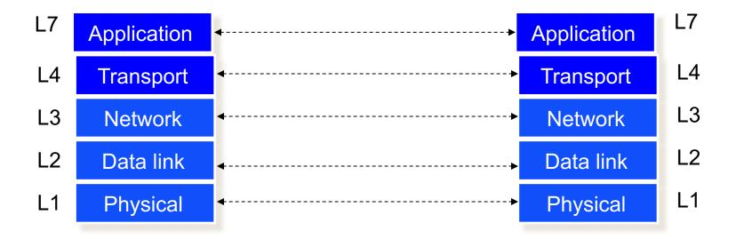
Communication between peer layers on different systems is defined by protocols
